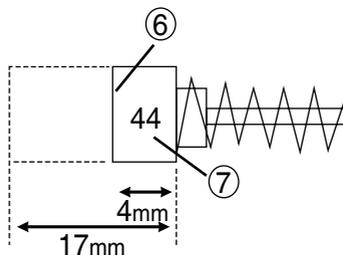
The carbon brush can be removed by removing the cap cover (9), cap rubber and brush cap in that order at the interior. To replace carbon brush reverse order of removal.
