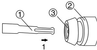
Put the bit into the hex housing and clamp the bit by turning the stop lever half a turn anti clockwise. This will lock the bit in place.
