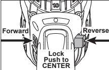
For **reverse** (counterclockwise) rotation, push in the control switch from the left side of the tool. **Check the direction of rotation before use.**
